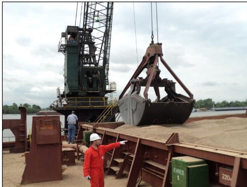
Figure 2: A crane loading pellets from a barge onto a ship (McNerney)
